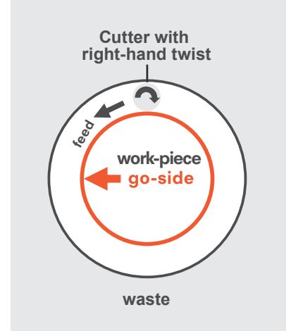
Cut shape = work-piece, feed in anticlockwise direction
