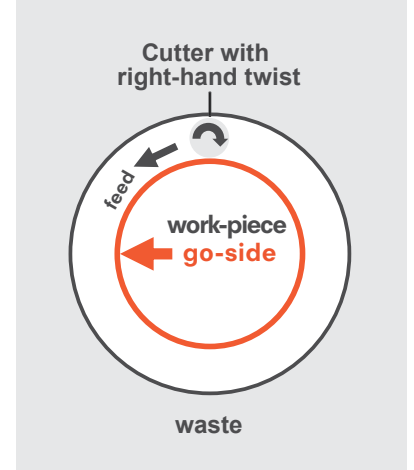
Cut shape = work-piece, feed in anticlockwise direction
